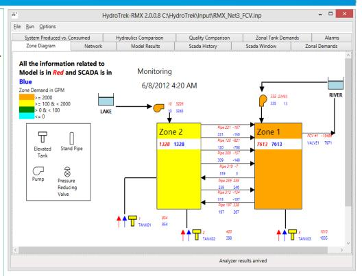
HydroTrek has the ability to display data in a number of ways to suit the needs of a utility. Individual components can be displayed (i.e. tank levels or pump flows), or the entire network can be viewed in terms of a zonal diagram displaying both SCADA and model values in real-time. HydroTrek output matches SCADA data because its algorithms accurately modify the model in real-time.
